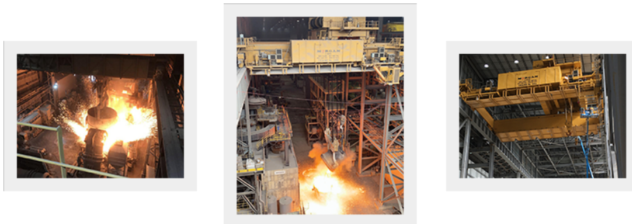
Morgan cranes at work. At times carrying more than 600,000 lbs. of metal in one load.
